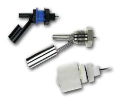
The operation of the Flowtechnik level probe for liquids LCSFS is based on the switching of a reed switch by a magnetic float, rotating around a fixed point or sliding along a stem.
