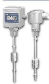
The operation of the LCSF100 level transmitter is based on the switching of reed switches by a magnetic float, moving alongside a protective tube, and the reed switches act on the elements of a resistor matrix, changing the total matrix resistance in linear proportionality with the level measured. In addition to providing a 2-wire 4...20 mA output signal with 6 or 12 mm level resolution, the transmitter may be equipped with up to 2 alarm contacts.
