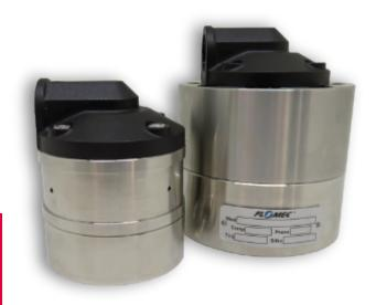
FLOMEC® OM Series, Small Capacity, High Pressure Flow Meters provide volumetric measurement of low flow, clean liquids up to 400 bar. Suitable for applications including metering lubricants, chemicals, grease, additives, and other high viscosity fluids.
