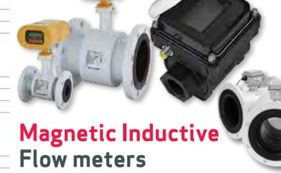
Containing no moving parts, magnetic inductive flow meters are ideal for polluted liquids or slurries. The straight through design also gives very accurate flow measurement over a wide span for many applications. If the liquid is conductive then this flow meter will measure it accurately. A wide choice of flow meter liners make this a popular choice in many process industries such as water treatment & foodstuff dosing or filling.
